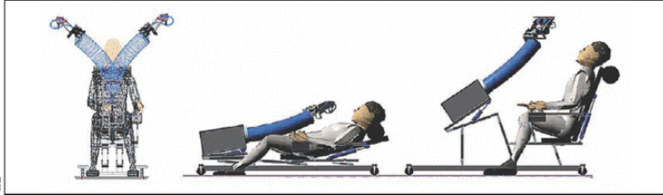
A belly chair in computer-simulated action. An EMMA's basic anatomy, minus any supporting structure, comprises an "actuation package" housing the pneumatic circuitry and cylinders array that power the arm; joystick controls; a mostly hollow polyurethane-cored arm that mimics the sophisticated motions of a human's (without the human's risk of injury); and finally, the "end-effector," onto which can be mounted sander, blaster, polisher, and/or vacuum, in single or ganged setups.
