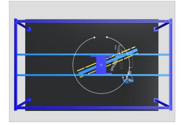
EMMA OMR Turret Systems traverse laterally on an X-Y frame, with rotational capacity provided by an integrated
