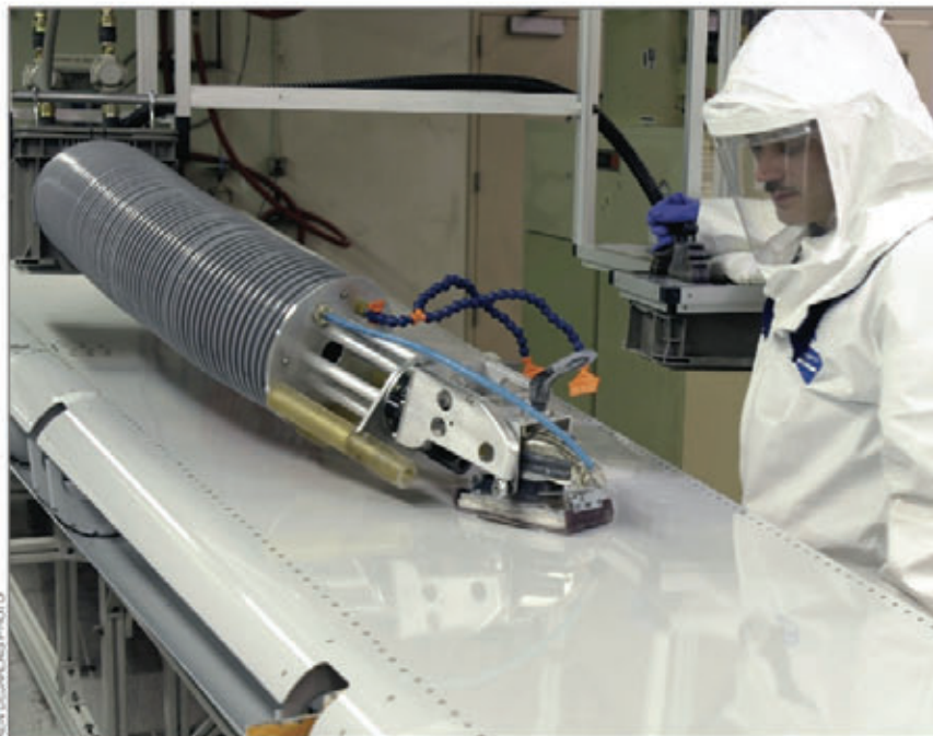
Dave Schaffer, paint lead in the 737 Rudder Paint shop in Renton, Wash., controls a new tool to sand rudders using a remote joystick. The new tool reduces worker exposure to soft-tissue injuries caused by vibrations during manual sanding operations.
